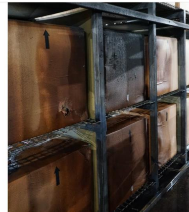
Figure 32: Charring, soot deposition, and water damage on northern target array
