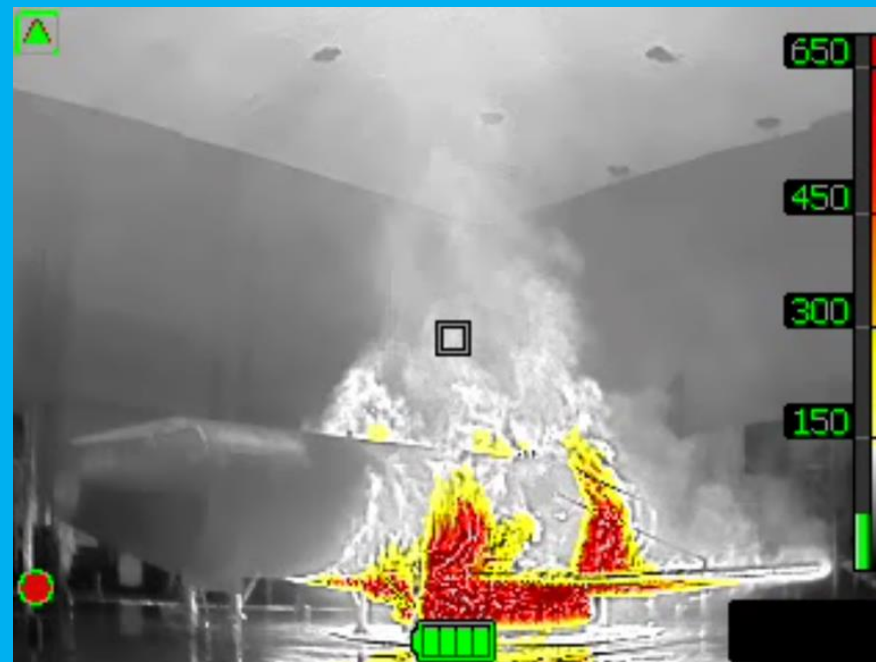
Fire developed 60 seconds after ignition – thermal view.
