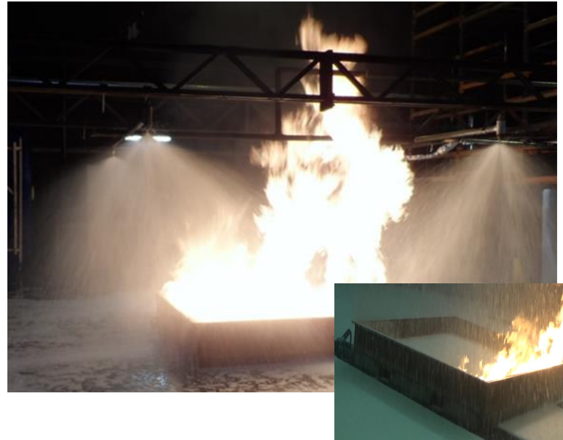
Sprinkler(Nozzle) fire test FM5130 & since 2022 VDS3896
