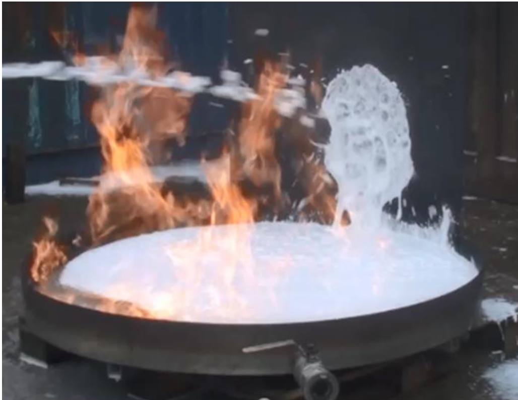
EN1568 fire test with a well foaming foam nozzle
